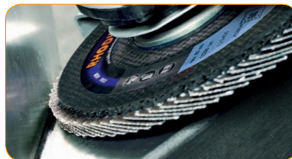
Inefficient, because most of the abrasive material remains unused.
